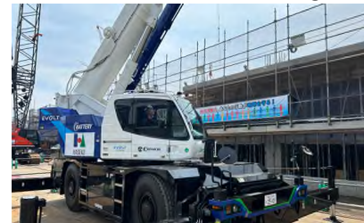
Adoption of battery-powered full-electrified rough terrain cranes
