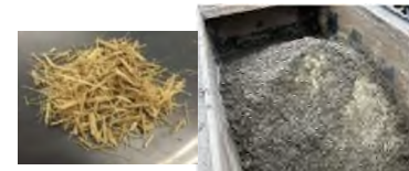
Joint development of construction sludge solidification technology using bamboo waste from Asuka Village with Fukuoka University (about 50% reduction in CO2 emissions)
