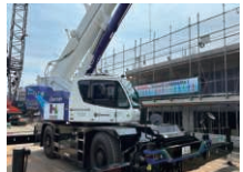
Adoption of battery-driven fully electric rough terrain cranes
