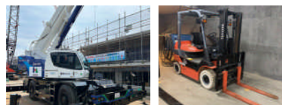
Adoption of battery-driven fully electric rough terrain cranes
