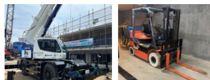
Adoption of battery-driven fully electric rough terrain cranes
